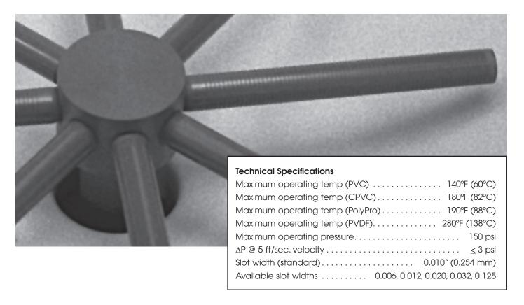
Safe Water Technologies standard PVC laterals are fabricated from Schedule 80 PVC pipe. Stocked diameters include 1/2", 3/4", and 1-1/4". Also available are pipe diameters of 1", 1-1/2", and 2". One end is threaded MNPT. The other end is closed with a flat end plug.
